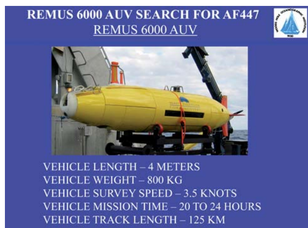
Figure 3: REMUS 600 AUV dimensions.
