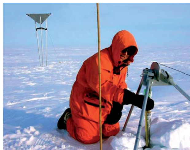
Figure 8. Here a neutron probe is lowered into a hole drilled in the ice. It collects essential data on snow and ice density layering to help understand the radar signals from the satellite and ultimately transform the height measurements into net change in ice mass, the main objective of Cryostat. Credits: Norwegian Polar Institute.
