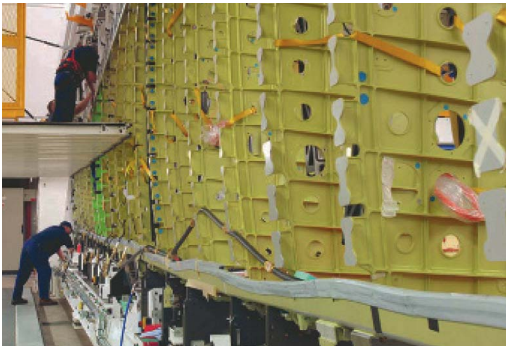
The A400M wing assembly jig.
