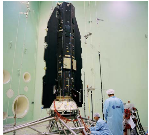
The GOCE Satellite in course of integration (Credit ESA)
